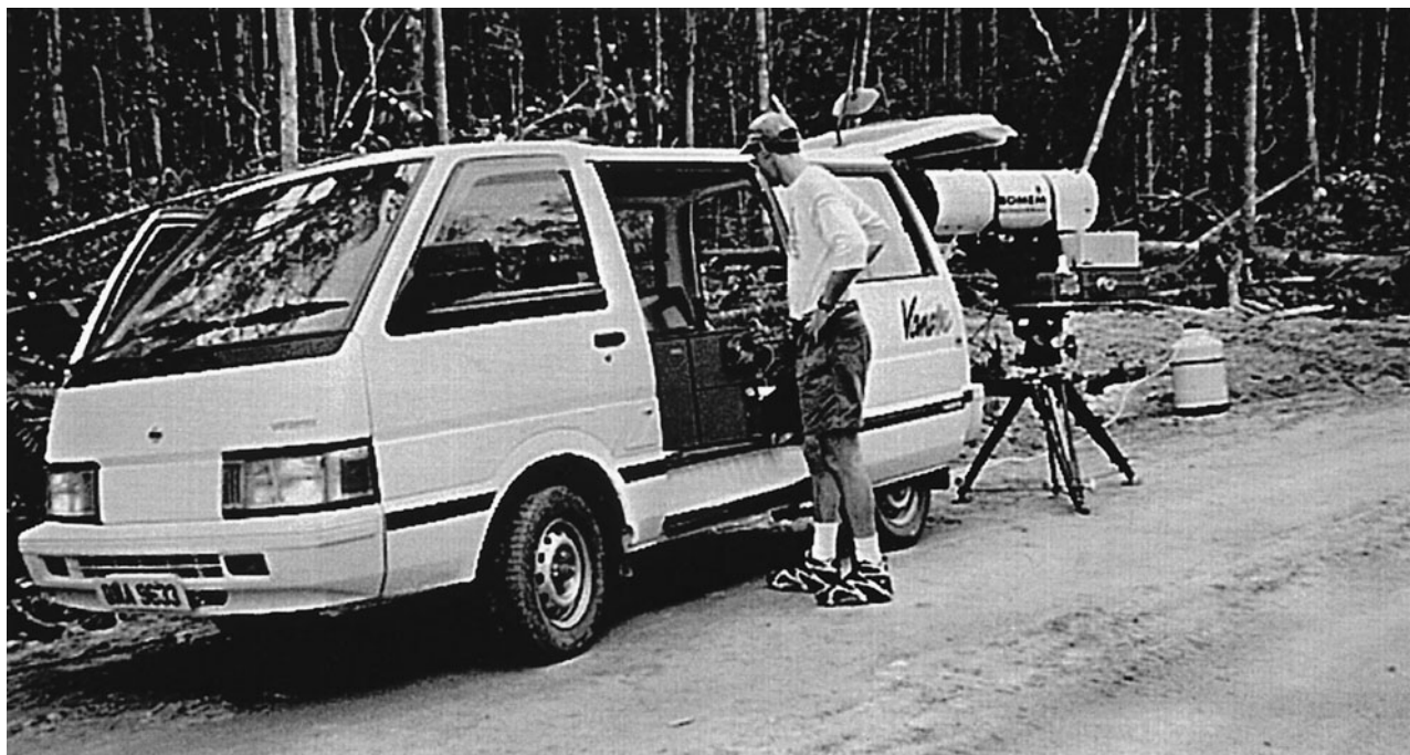
Figure 3. Volatile organics analysis in the Malaysian jungle with a transportable GC-MS and a transportable long-path reflective FT-IR.
