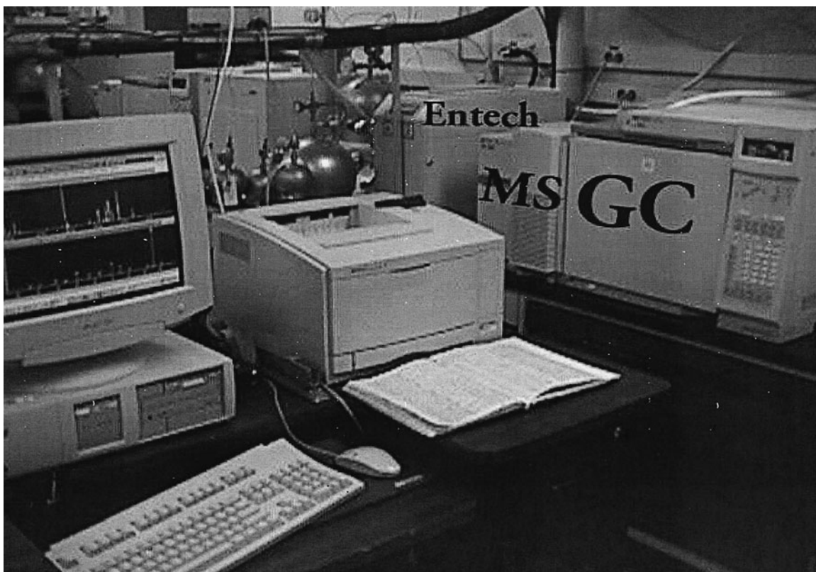
Figure 8. Photograph of analytical system used for ground-based GC/MS analyses of VOCs in archival samples of cabin atmospheres.
