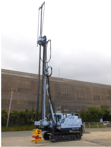
Fig. 4 Construction Machine: single mixing shaft machine for DMM
