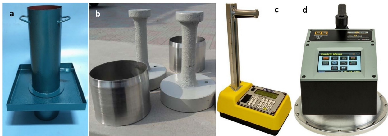
Fig. 3 Device for detecting density. a sand-cone cylinder. b cutting ring. c nuclear density gauge. d non-nuclear density gauge
