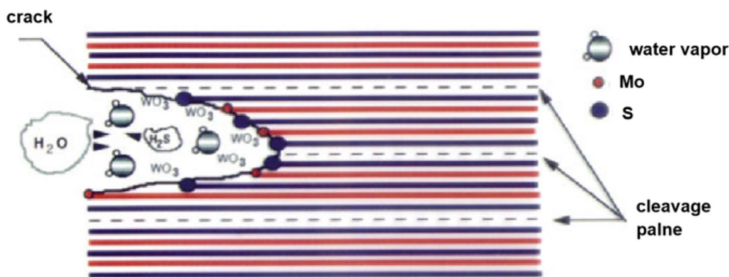
Fig. 10 Schematic representation of the reaction mechanism of MoS 2 films with water [18]. (c) reproduced from ref. 3. Copyright ©2012 J Mater Sci
