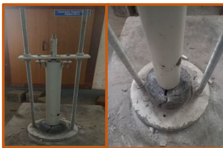
Fig. 2 Impact test apparatus and test specimen
