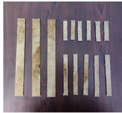
(b) FLAX/PLA/EPO composite specimen as per ASTM Standard
