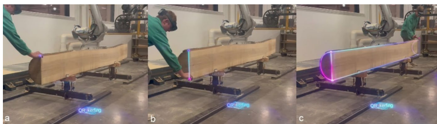
Fig. 5 Object localization is used to determine the work object placement for robotic fabrication
