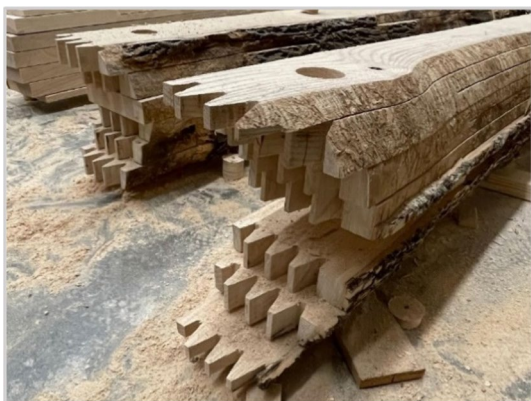
Fig. 12 Robotically Kerfed logs with finger joints and threaded rod holes
