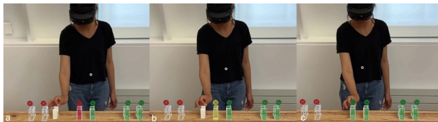
Fig. 16 Object calibration is employed to ensure the hex nut locators are adjusted to match the digital model. As the physical hex nut locator moves closer to its digital position, the notation would transform from red to yellow to green
