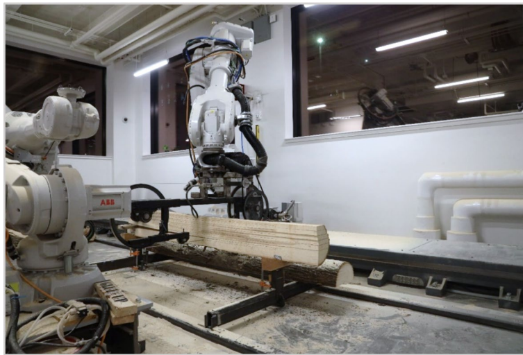
Fig. 9 6-axis robotic arm with a 5hp bandsaw end-effector cutting a log after object localization
