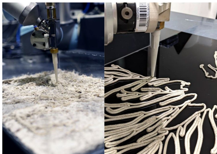
Fig. 9 Image showcases the mixture of agricultural waste including mycelium, coffee grinds, paper pulp and hemsps seeds being extruded from the Universal-10 robot
