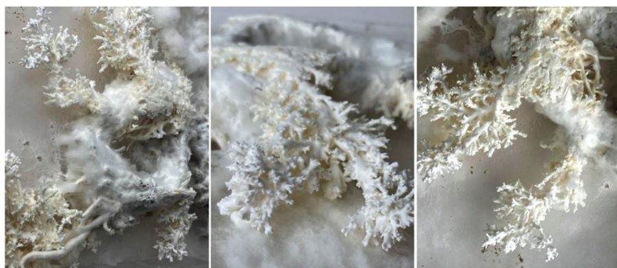
Fig. 11 Clay infused with mycelia robotic extrusions. Overtime, the mycelium began to grow from the organic mixture and wandered around the surface area in search for additional nutrients
