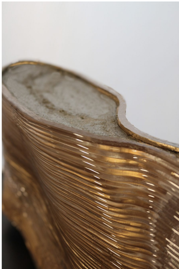
Fig. 15 Sacrificial Formwork prototype: fibre-reinforced concrete is cast into a 3D printed polymer skin
