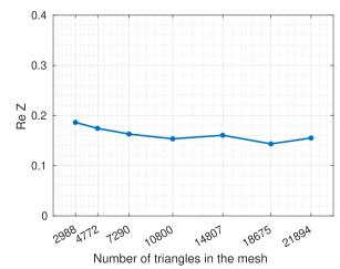
Fig. 9 Impedance values for different mesh sizes as calculated by Adamant
