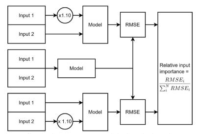
**Fig. 7** Schematic of how the relative input importance is calculated. Note that there is also a -10% variation for all parameters that is not depicted here, and that  $RMSE_i$  would actually be the RMSE of both +10% and -10% summed for each input parameter
