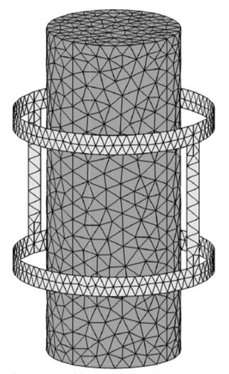
Fig. 8 Mesh of the plasma computational domain with the Nagoya III antenna
