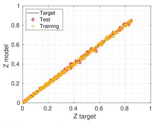
Figure 14 shows a distinctly different correlation to the decision tree and the ensemble. It is clear that the SVM fails to accurately predict both the training set and the test
