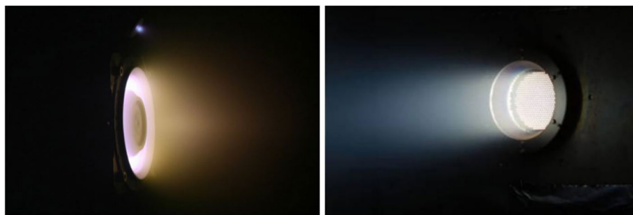
Fig. 8 (Left) PPS1350-TSD operating with N 2 /O 2 mixture (305 V, 2.75 mg/s); (right) RIT10 thruster operating with O 2 . Extracted from [115]
