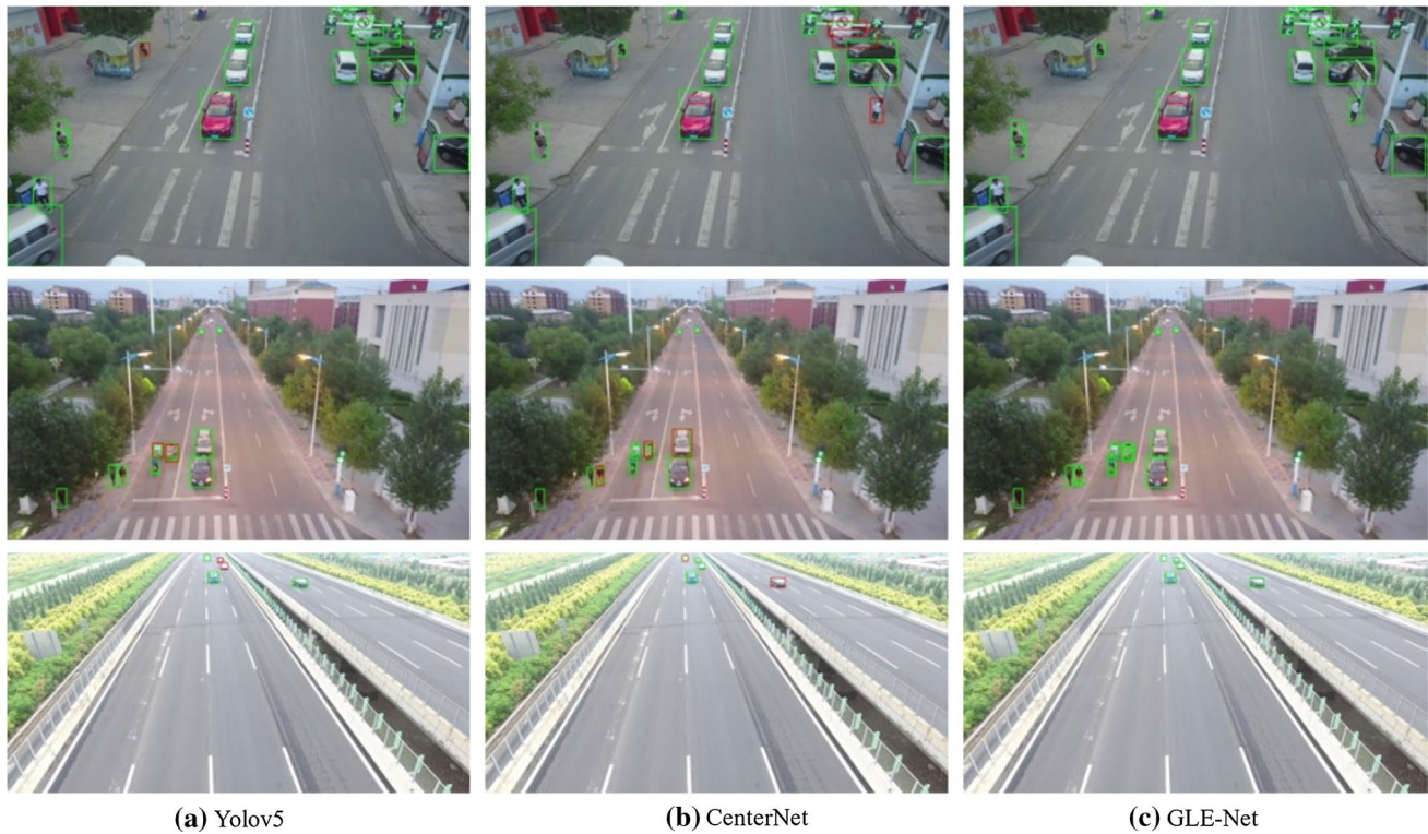
Fig. 7 Qualitative results of Yolov5, CenterNet, and GLE-Net in aerial images. The red boxes denote undetected objects, and the green boxes denote detected objects
