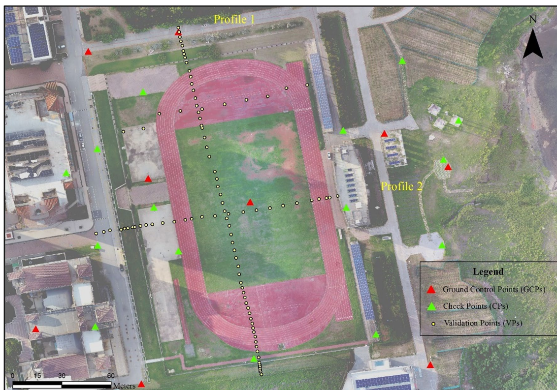
Fig. 3 Experimental flight field map. The red triangles are the 12 GCPs; the green triangles are the 15 CPs; the yellow circles are the terrain VPs
