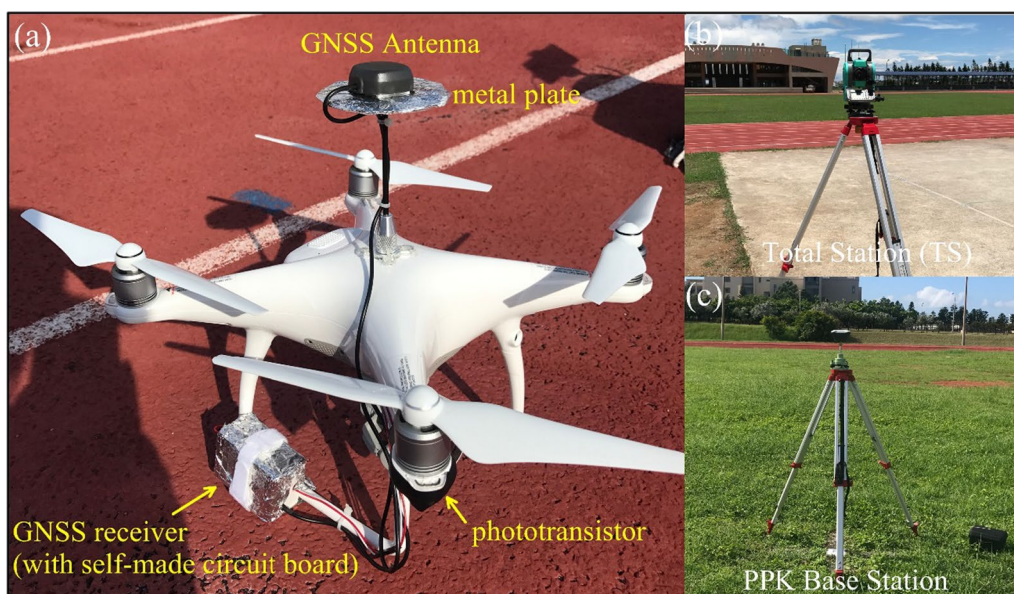
Fig. 1 Images of the research equipment. a Self-made UAS-PPK system (components include a self-made circuit board, a GNSS receiver, a phototransistor, and a GNSS antenna); b Total station for surveying; c PPK base station
