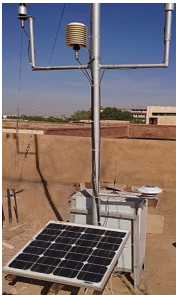
Fig. 4 Wind and solar measurement station- ERC rooftop
