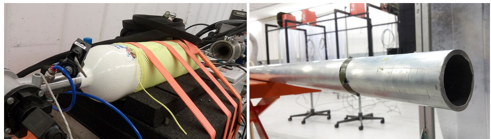
Fig. 3 The low-pressure launcher originally used for the first few tests located at the Royal Military Academy in Belgium. The launcher was a pneumatic assembly capable of reaching 0.4 MPa (145 PSI) and included a 1925 mm long and 50 mm diameter barrel
