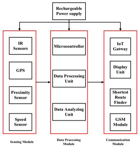
The flow chart of smart routing system is shown in Fig. 8. The flow chart describes the automatic "chalan" system for over speeding also vehicle tracking and information sharing with traffic department. If the driver is sleeping or his eye is closed for more than 5 s, the vehicle stopped will be automatically slow down and automatic breaks will be applied.
