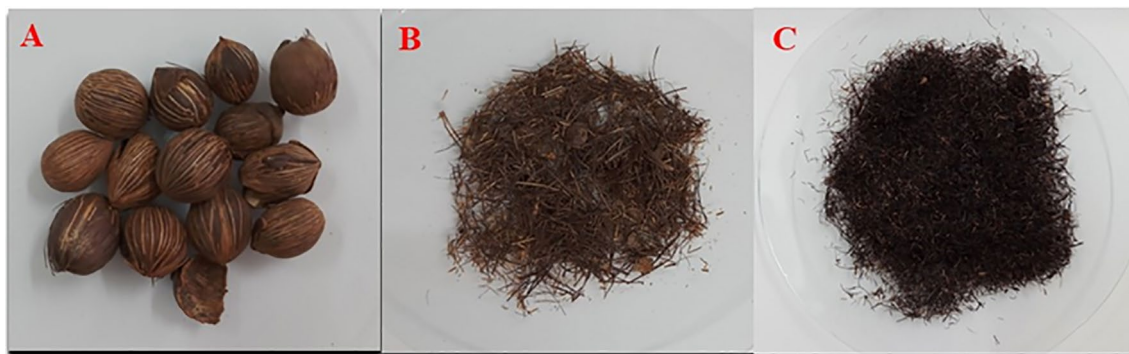
Fig. 2 a Oenocarpus bacaba Mart fruit, b in natura Oenocarpus bacaba Mart fibers, and (c) Oenocarpus bacaba Mart fibers after alkaline modification
