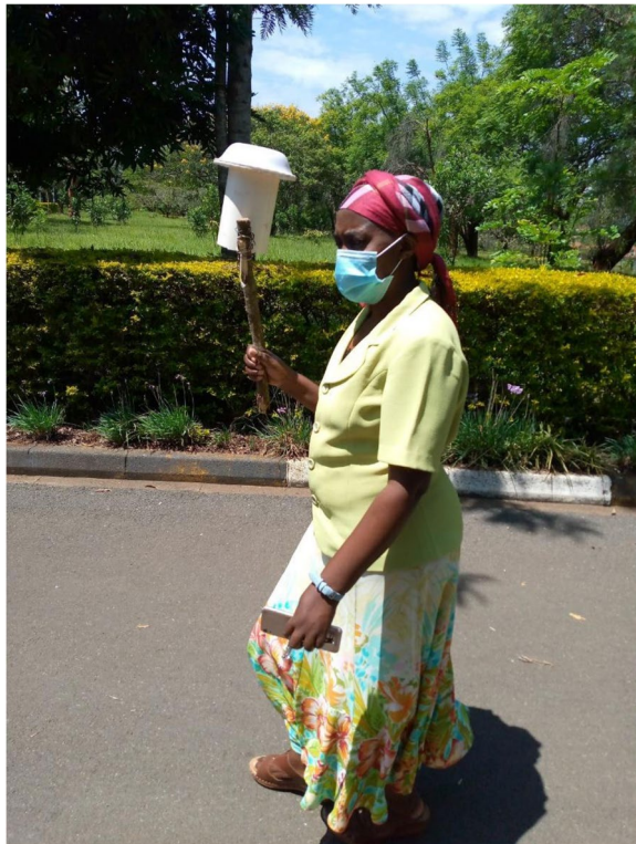
Fig. 4 A fabricated (‘rocket type’) radiation shield containing the Hobo Pendant temperature logger that was used in traverse walk around campus. The radiation shield was developed from 160 mm PVC pipe and white melamine bowls
