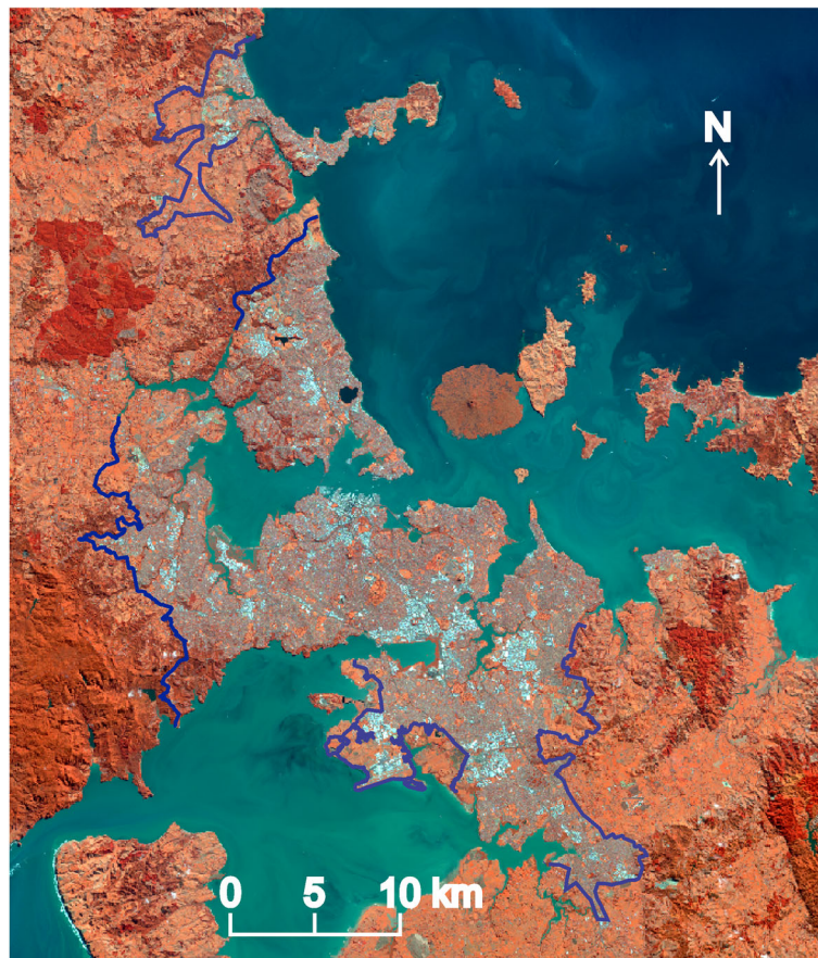
Fig. 2 Subset color composite of bands 5 (red), 3 (green), and 2 (blue) of Landsat 8 OLI image recorded on 14 April 2014 (size: 2136 by 1833). It clearly shows urbanized areas (e.g., industrial areas in blue and residential areas in reddish blue). Blue line: metropolitan urban limit
