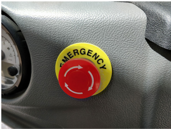
Fig. 15 The emergency button for safety consideration
