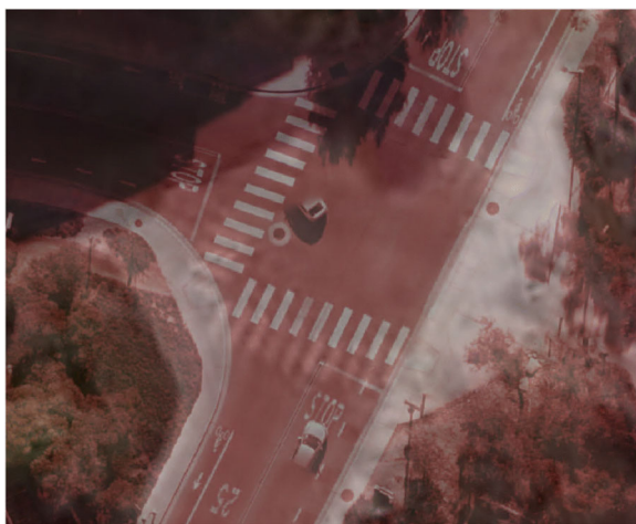
Fig. 38 Semi-transparent overlay of UAV captured, geo-referenced orthomosaic image data over Google satellite imagery of intersection at the UC San Diego engineering campus. Inconsistencies of pedestrian crossings emphasize the issues associated with geo-referencing, and temporal data agreement, in addition to strong scale differences
