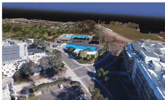
Fig. 36 UC San Diego engineering campus 3D point cloud from geo-referenced UAV imaging
