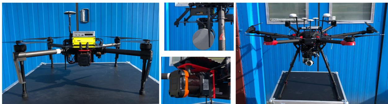
Fig. 9 Experimental platforms: DJI Matrice 100 equipped with a Hokuyo UTM-30LX LIDAR sensor (left), DJI Matrice 600 Pro equipped with a Velodyne Puck LIDAR sensor (right)
