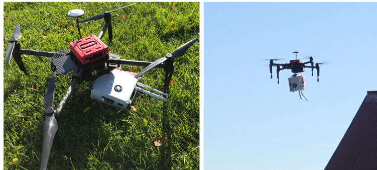
Fig. 10 The DJI Matrice 100 system with a CommKit attached
