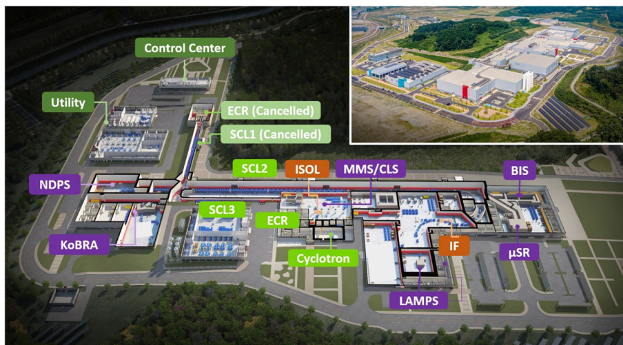
Fig. 1 Layout of the overall RAON facility. The items written in green and brown are the accelerator systems and RIB production systems, respectively. The items in purple are the experimental setups. One of the low-energy superconducting linac SCL1 and the associated ECRs were canceled because of the budget shortage, and the SCL3 and another set of ECRs play their role instead. The small panel in the upper-right corner shows the recent bird's-eye-view image of the RAON area
