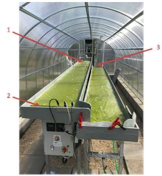
**Fig. 2** General view of the thin-layer cascade used for the experiments. Measurements of the main physico-chemical variables (dissolved oxygen concentration (DO), pH, and temperature) were performed in three points of the culture system, (1) 20 cm from the culture inlet, (2) in the channel connecting the two culture lanes, and at the end, i.e., 5 cm before the culture falls into the retention tank. Culture probes (pH, T, DO) were placed in the channel (3) connecting the two lanes
