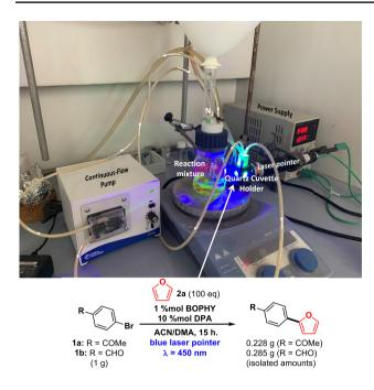
**Fig. 6** Photograph of the setup of the home-made continuous-flow photochemical device for the gram-scale arylation of furan photocatalyzed by **TFU** technology
