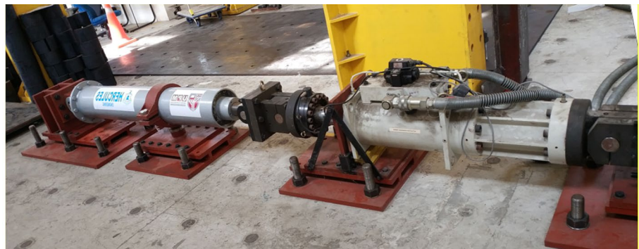
(a) Experimental test setup for RBD device
