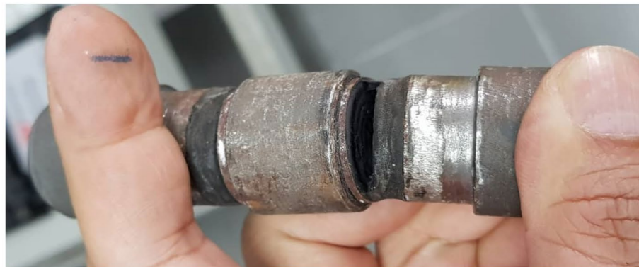
(c) Deformed and teared rubber specimen
