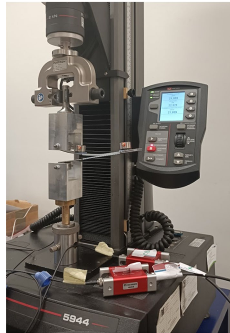
Fig. 4 Proper DCB tests were conducted using INSTRON 5944
