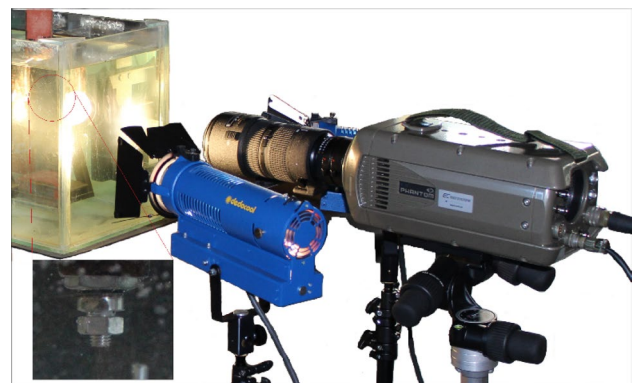
Fig. 2 The stand for assessing water jet properties (including a zoom view of self-excited water jet head)
