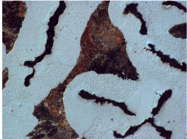
microstructure: compacted graphite, ferrite, pearlite
