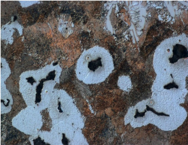
microstructure: compacted graphite, pearlite, ferrite, cementite
