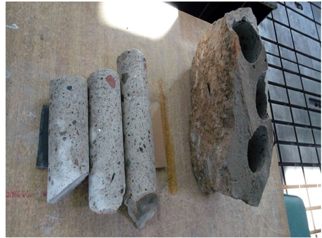
Fig. 16 Concrete probes taken
