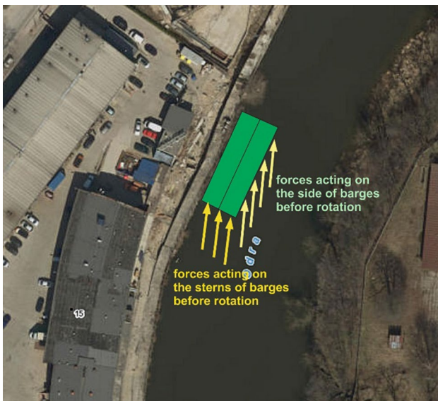
Fig. 21 Forces acting on the sterns and sides of the barges before rotation [photo: https://geoportal.wroclaw.pl/ ; 15.03.2021]
