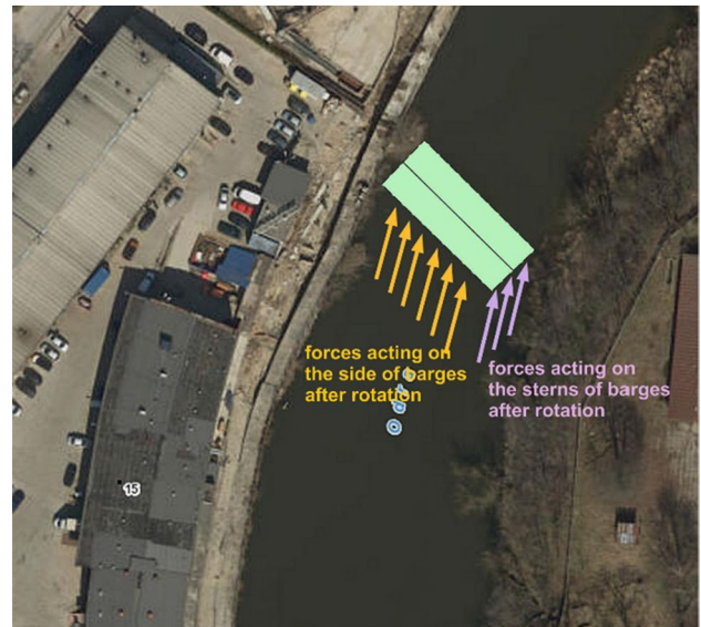
Fig. 22 Forces acting on the sterns and sides of the barges after rotation [photo: https://geoportal.wroclaw.pl/ ; 15.03.2021]
