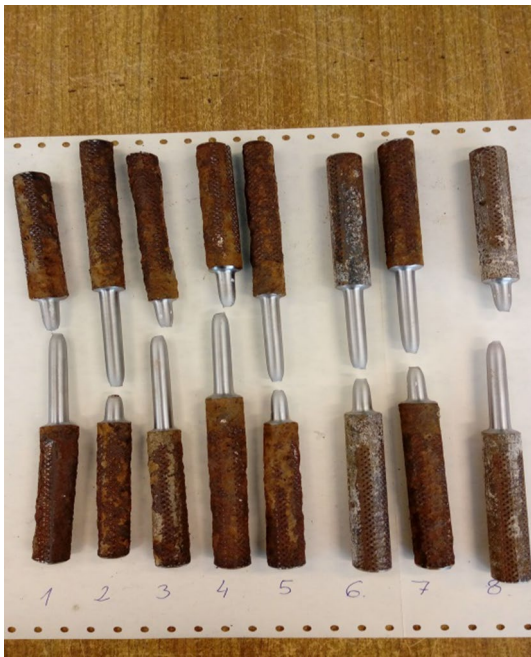
Fig. 18 Steel rebar probes after testing
