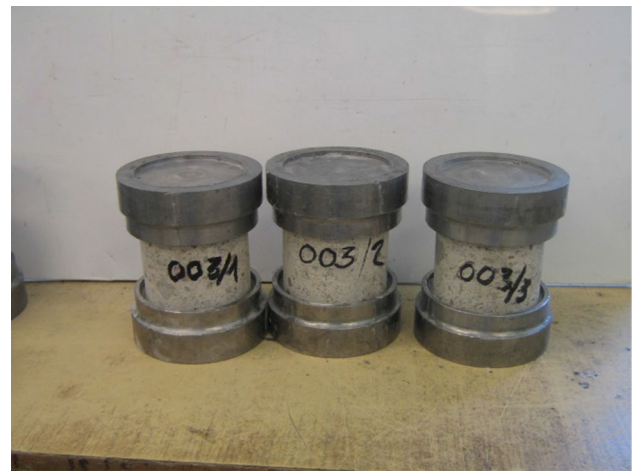
Fig. 17 Concrete probes prepared for testing
