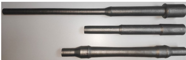
Fig. 18 Examples of parts rolled in a CNC skew rolling mill
