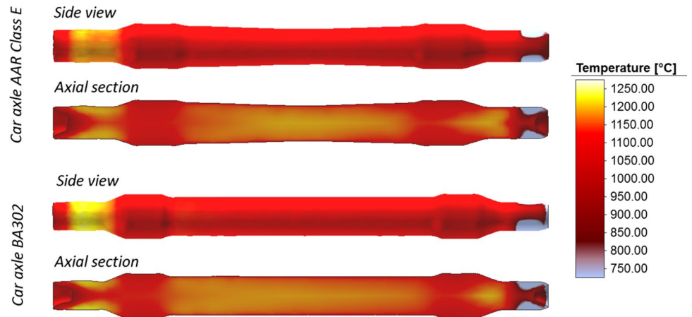
Fig. 12 Temperature distribution in rail car axles produced by skew rolling in the CNC rolling mill
