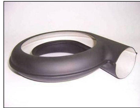
Fig. 3 “Compressor scroll. The final shape produced by PALBAM-AMTS”, Reprinted from MAGFORMING Development of new Magnesium Forming Technologies for the Aeronautics Industry, by Henn and Fein [24], Copyright 2010 by MagForming Consortium. Reprinted with permission
