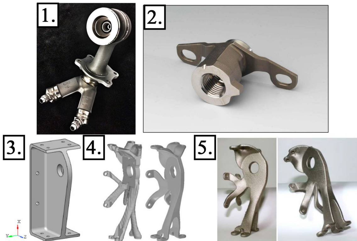
Fig. 6 Examples of aerospace parts manufactured by SLM technology. (1) “A 3D printed fuel nozzle made by General Electric Company”, Reprinted from Additive manufacturing at GE Aviation, 2014, GE Reports, Copyright by 2014 General Electric. (2) “Additive manufactured boroscope boss”, Reprinted from In-Process Control of Selective Laser Melting by Quantitative Optical Tomography by J. Bamberg, et al., 2016, 19th World Conference on Non-Destructive Testing 2016, Copyright by 2016 Creative Commons. (3) “Original
