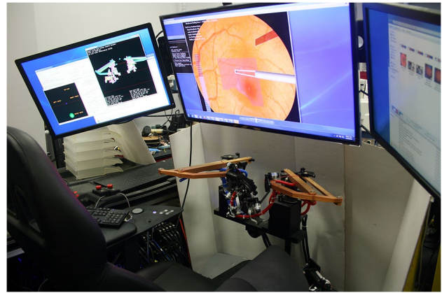
Fig. 3 Shown is a photograph of a prototype of an immersive, augmented-reality surgical “cockpit” created at UCLA for the purpose of testing the feasibility of using such a system in robot-assisted retinal surgery. (Reprinted by permission from Springer Nature from: Gerber MJ, et al. Eye (Lond) . 2020 Sep; 34(9): 1554–1562. https://doi.org/10.1038/s41433-020-0837-9 ) [28]
