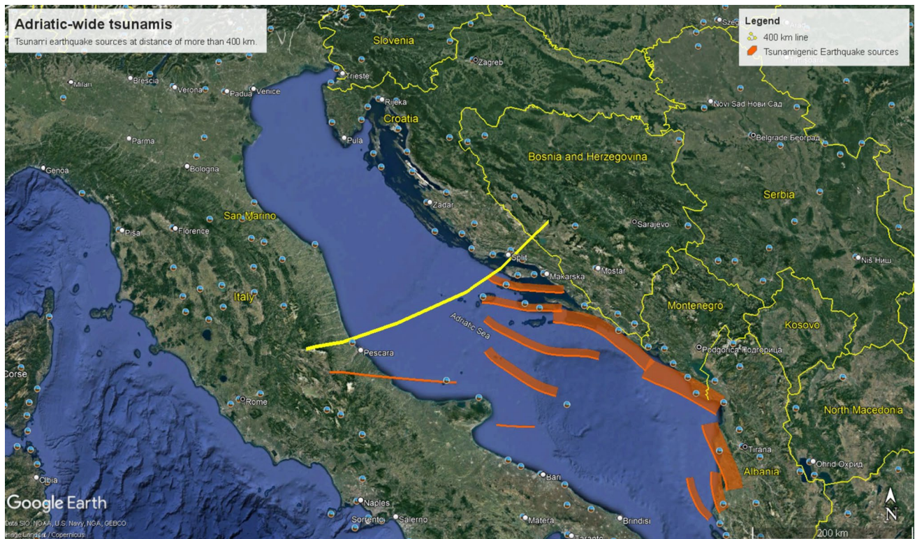
Fig. 5 Tsunamigenic earthquake sources at Adriatic-wide scale (distance from the AOI is > 400 km). The yellow line defines the sources at more than 400 km, while red rectangles are the tsunamigenic sources
