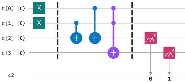
Fig. 6 Quantum adder circuit
