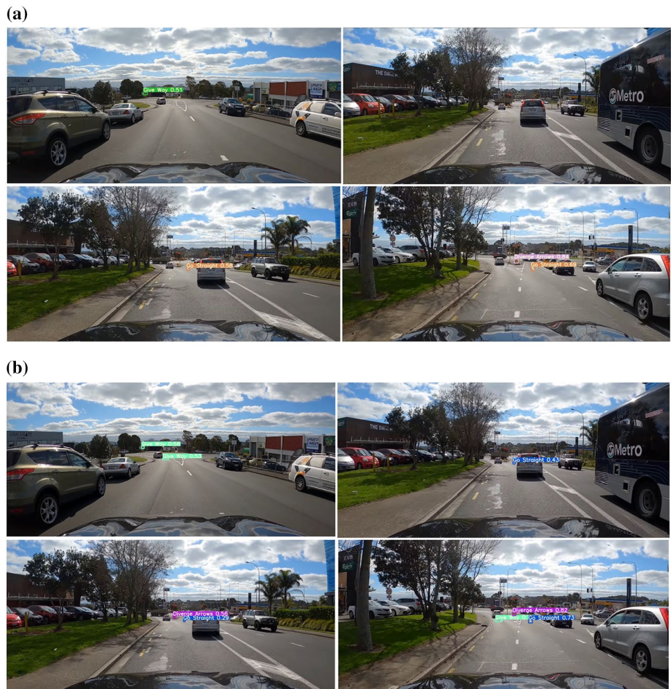
Fig.12 The result of recognition on FRIDA dataset with YOLOv5 (a) and Faster R-CNN (b)
