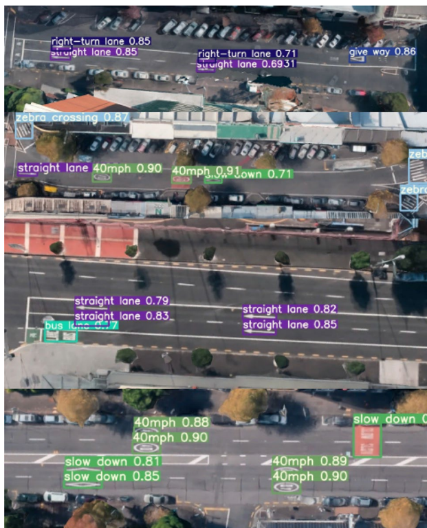
Fig.19 TSR results with satellite images
