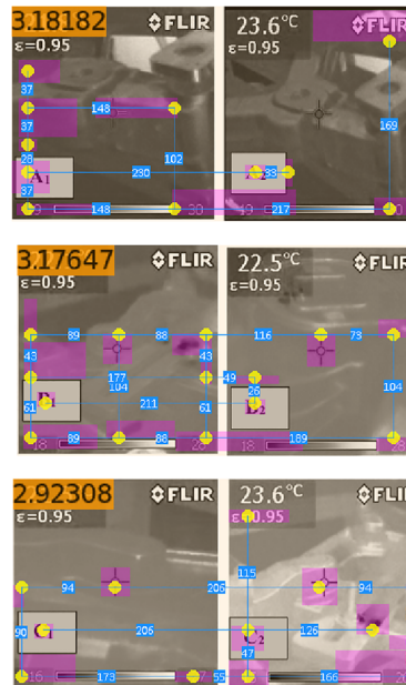
Fig. 19. Temperature measured in SD1, SD2 and SD3 corresponding respectively to A1, B1 and C1 (with index 1 and 2 denotes the temperature state before and after measurement) during the hysteresis testing at fixed frequency of 0.35 Hz.
