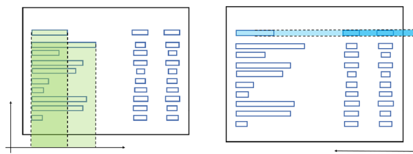
Fig. 7 Row, column grouping through projection on X and Y axes
