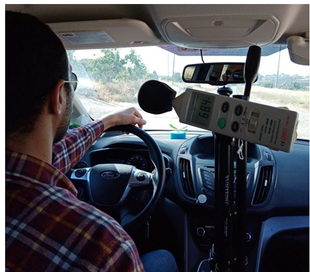
Fig. 1 Set-up and mic position for interior noise measurement [17]
