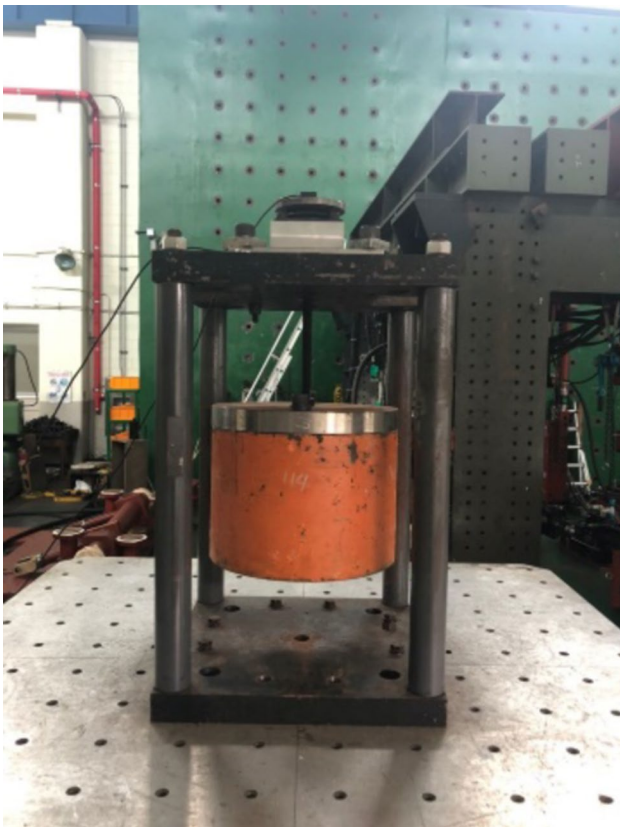
Fig. 9 Dynamic test for the rubber mount
