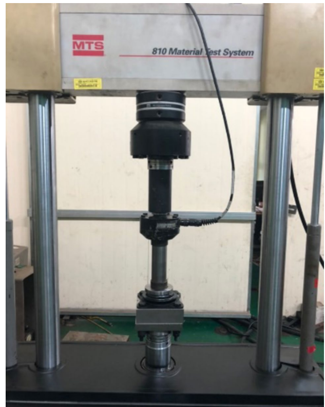
Fig. 10 Static stiffness test for the rubber mount
