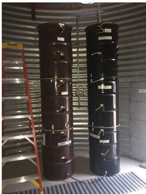
Fig. 2 Columns of barrels used to test potential phosphine distribution deeper into the corn grits. The columns had air sampling ports located vertically at every 40 cm from the top of the corn grits
