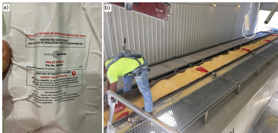
Fig. 1 Photo of phostoxin prepack (a) and photo of top of railcar (b) with corn grits for shipment and the Centaur sensing units were placed on the top in red bags
