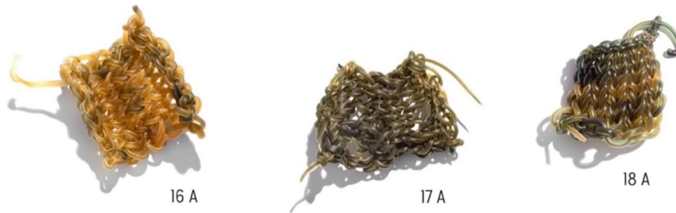
Fig. 12 Alginate-based Bio-yarns knitted: Sp. Bio-yarns from Experiments 16A/17A/18A of Table 3, based on dye bath obtained by liquid dye first filtration, selected blue-green leftover bath from
