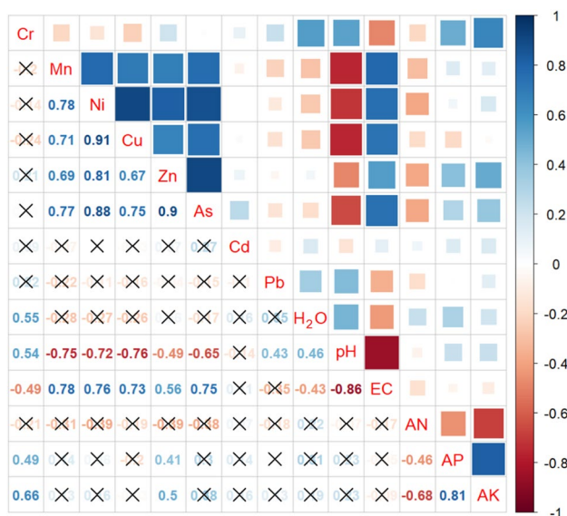
Fig. 6 Pearson correlation between the F4 fractions of potentially toxic elements and soil properties. H 2 O soil moisture, AN ammonium nitrogen, AP available phosphorus, AK available potassium
