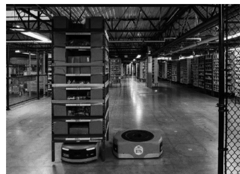
Fig. 1 RMFS with mixed shelves and picking station (accessed via amazonrobotics.com).
