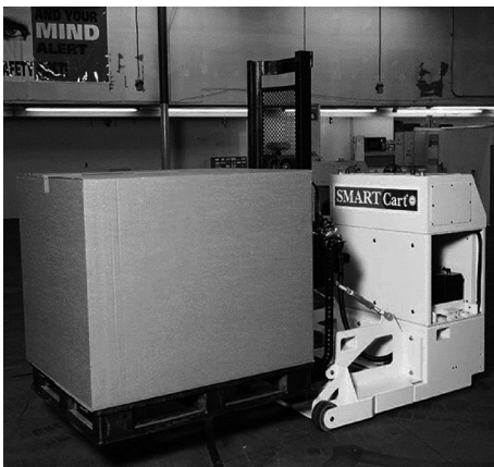
Fig. 8 AGV-assisted order picking (accessed via directindustry.com/prod/crown/product-9227-1769803.html ).
