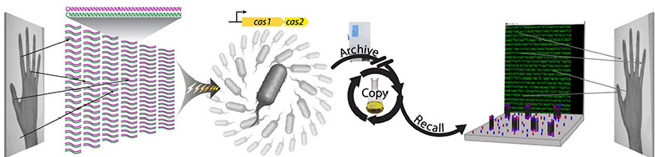
Fig. 13 Flowchart showing CRISPR-based DNA storage technology (Shipman et al. 2017)
