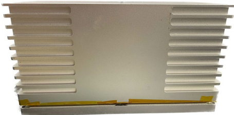
Fig. 10 Closed cube to create convective conditions as similar as possible to those on the ISS
