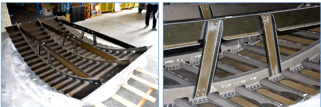
Fig. 1 Section of interest of the commercial aircraft fuselage trunk (left) with a focus on the test article (right) [19]
