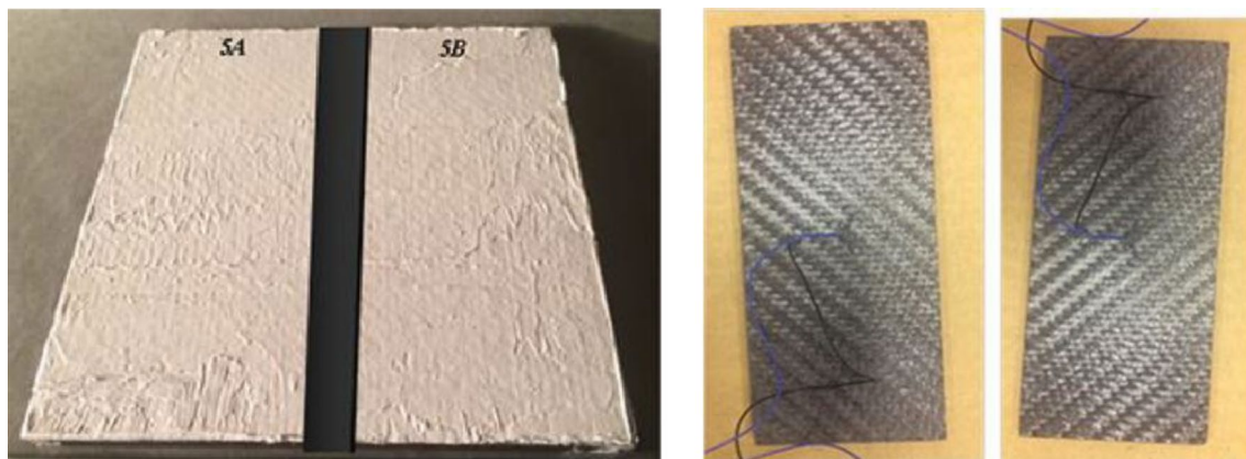
Fig. 1 A square tile cut out from commercial C/C slab, split in half for the thermal characterization: coated surface (left), back surface (right)
