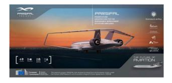
Aiming to demonstrate the technical, environmental and economic feasibility of a box-wing configuration, the project has been focused on the needs of short-to-medium routes air traffic (< 4000 km), for which most of the aircraft in service today belongs to category "C" of the ICAO reference code of airports (wingspan within 36 m).
