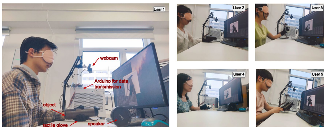
Fig. 8 Actual use scene. The main hardware of our system is marked in User 1's picture. When the mouse is clicked, the system begins to work. The webcam and glove are turned on at the same time to collect data. The blindfolded user then repeatedly changes the posture of his gloved hand to grasp the current object to build his own cognition of the item and give his own judgment. When the collection is done,
